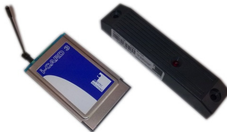
Fig. 1. RFID interrogator and transponder used in the research ( i-Card III interrogator (left) and i-Q transponder (right) of the Identec Solutions long range active RFID system)
